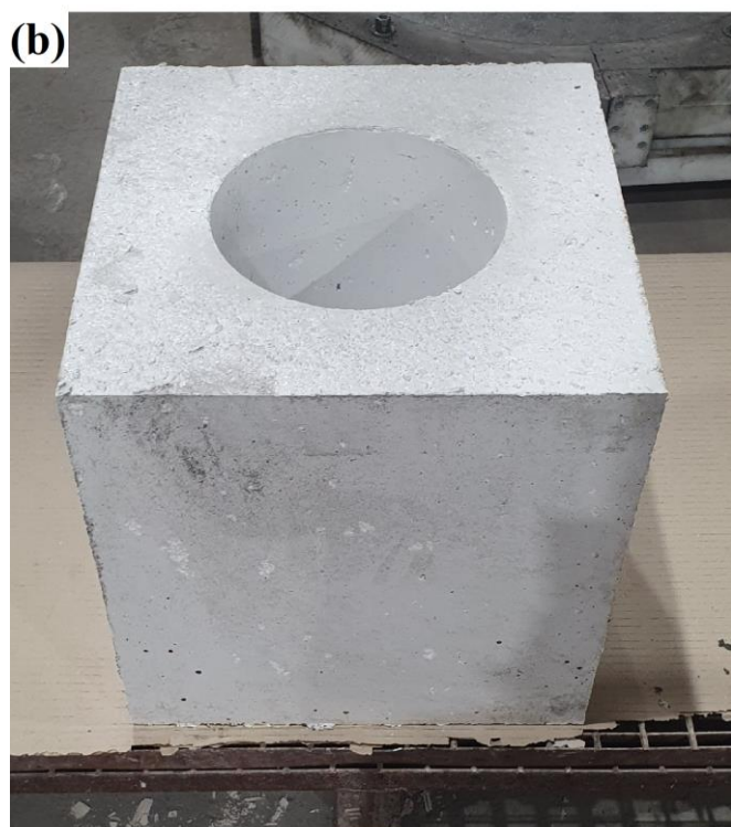
Figure 4: Well block casted from NCC-P mass (a), NCC-P well block after demolding (b)
